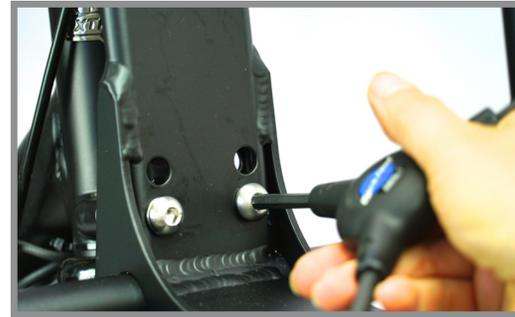
**Step 4:** Tighten all four bolts smoothly and evenly, alternating in a criss-cross pattern. Tighten them to 6-10 N-m
