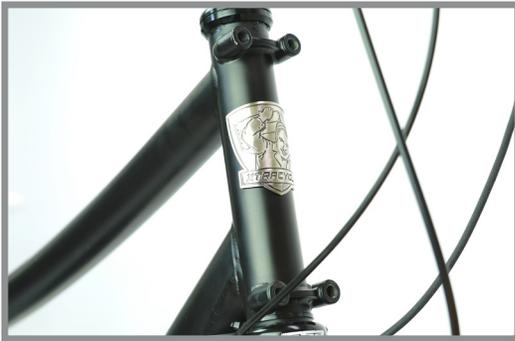
**Step 1:** Determine the appropriate mounting holes for your PorterRack by holding it up against the head tube bosses.
