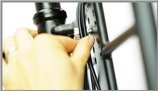
**Step 3:** Slide each M8 bolt through a spacer and thread it into its head tube boss a couple of turns while holding the PorterRack in place.
