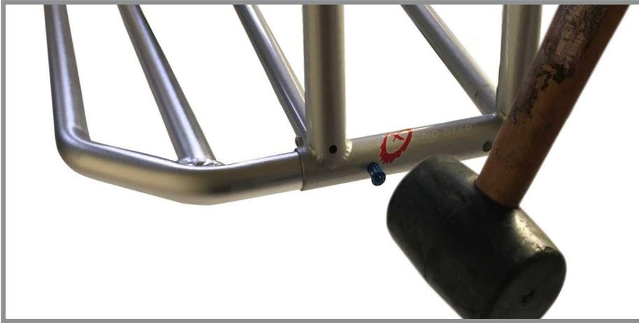
**Step 2:** Insert anchor into lined up hole. Using a mallet, push anchor until it is flush with Xtracycle frame.
