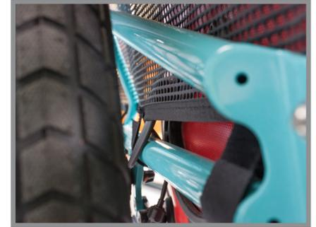
Pannier hooks attach to the P-Rail in the same way that they mount to a traditional bike rack. This works especially well for attachments that have a safety catch built into the hook itself.
