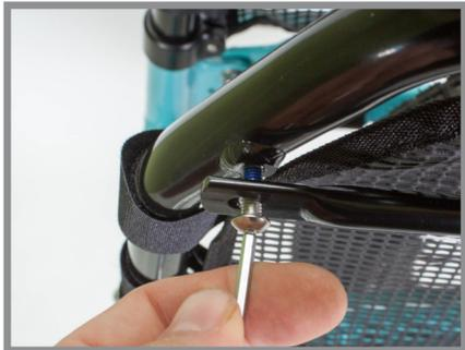
**Step 2a:** Loosely fasten one of the eyelets to the V-Rack, using an M5 bolt. As before, leave enough play for the rack to move around.
