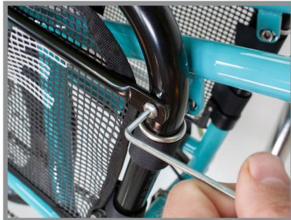
**Step 2b:** Install the third M5 bolt on the other side of the rail. This time tighten it all the way, then proceed to tighten the other bolts.
