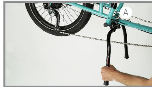
**Step 3b:** Put the legs into the down position and pull them towards the front of the bike to ensure that the KickBack is rotated as far forward as possible and centered on the boom tube (A).
