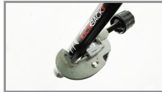
**Step 5c:** Cut each leg where appropriate. A pipe-cutter is the easiest solution, but a hacksaw and clamp-on guide will also work.
