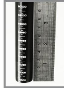
If you're installing on another Xtracycle or want to fine tune things, measure up the distance you calculated in Step 4c from the bottom of each leg and mark that location to cut.
