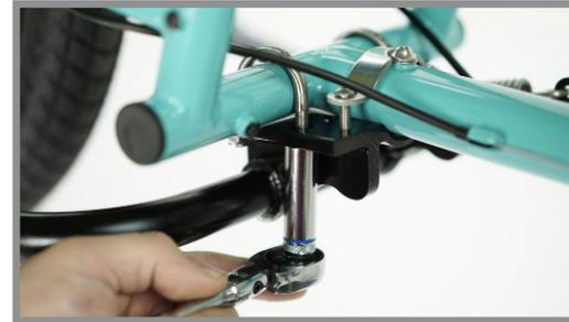
**Step 3a:** Moving the legs as necessary, lightly snug all four nuts with a 10mm socket wrench. Alternating between nuts can keep the KickBack from pulling to one side or the other.
