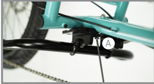
If your Xtracycle has a threaded boss on the underside of the boom tube (A), just ahead of the front bridge: start to thread one m5 bolt into it far enough to keep the KickBack attached to the frame. Do not tighten.
