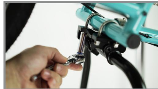
**Step 3d:** Torque all four nuts to 6 Nm.
