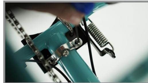
**Step 3c:** Tighten the M5 bolts on the BoomStrap or the single M5 bolt below to 3Nm.
